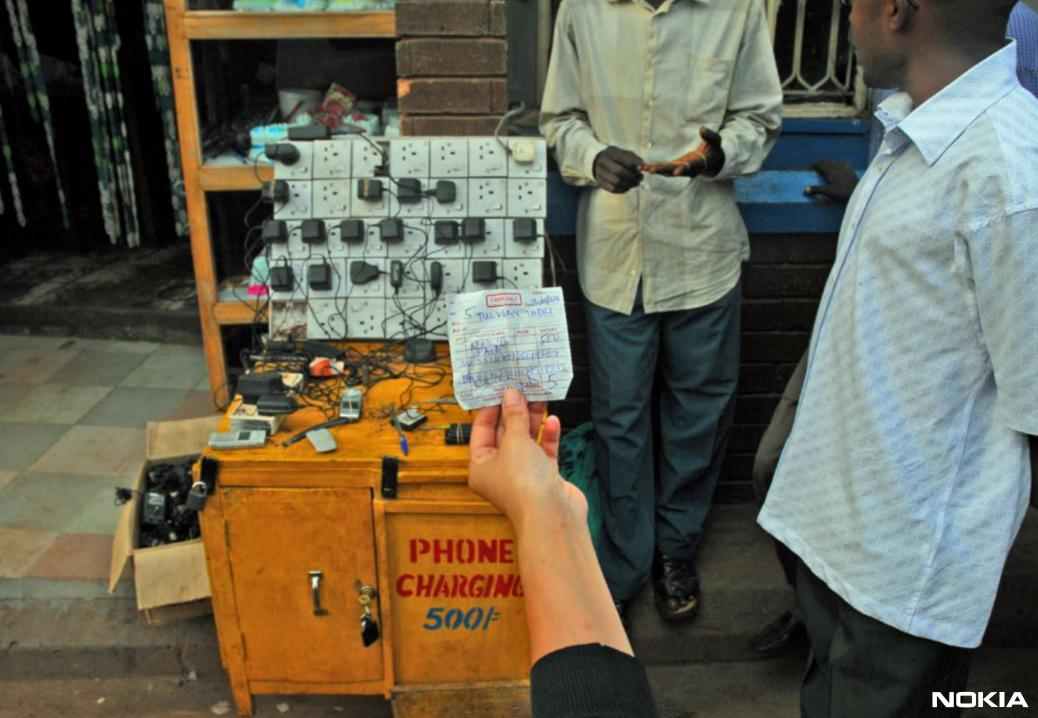
Charging cables are threaded though to a secure storage space Batteries can also be charged without the phone being present
